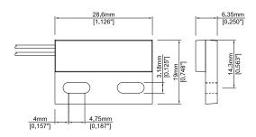
Reed Sensors with Mounting Holes for Screw Fastening
