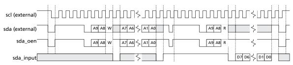
To accomplish an 2-wire interface read transfer, the host must perform the following steps:
