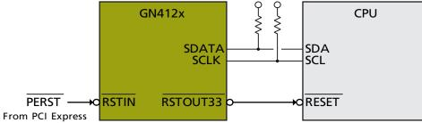
**Note:**Note: By default, the GN412x will respond to a 2-wire address of 5 ("101"). More information on the 2-wire interface controller is found in 7.1 2-Wire Interface.
