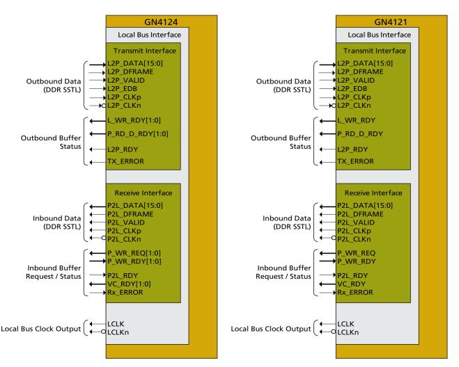
The local bus interface of the GN412x is composed of two primary sets of high-speed signals:
