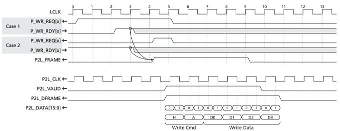
The write command shown in Figure 5-3 consists of a 32-bit header (H), followed by a 32-bit address (A), and concluded by a burst of 4 x 32-bit data transfers.
