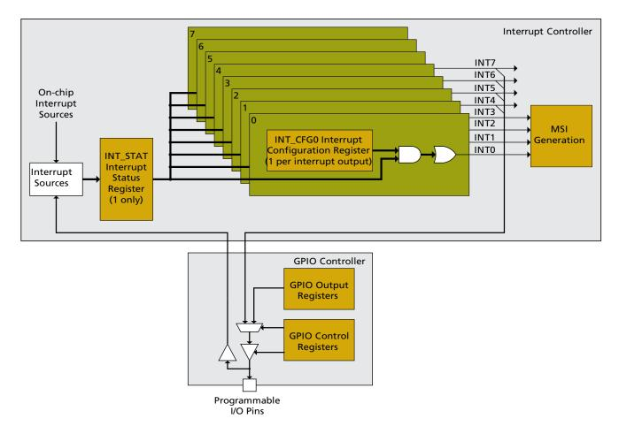
Figure 6-1: Interrupt Controller Block Diagram
