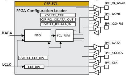
To support both Altera and Xilinx devices and to support future changes to the configuration protocol, FPGA configuration is initiated via SPRI GPIO pins. The control signals shown in Table 8-1 are required to program Altera Cyclone and Xilinx Spartan-3 devices.
