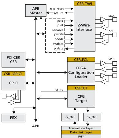
Figure 7-1: APB and Peripheral Devices Block Diagram.
