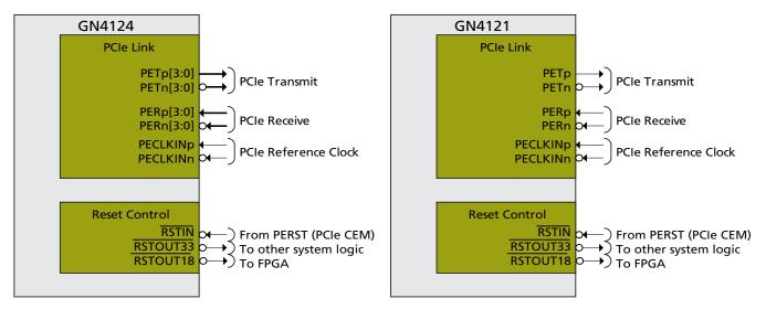
PETp/n[3:0] and PERp/n[3:0] are the high-speed transmit receive pairs for the 4 lanes of the GN4124 PCI Express interface. A 100MHz differential reference clock is also used (PECLKINp/n).
