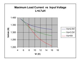
Figure 2. Theoretical maximum load current curves.
