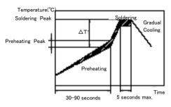
[Allowable Soldering Temperature and Time]
